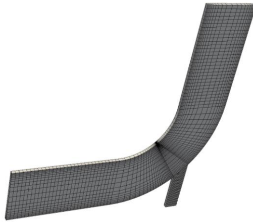
The Hex Fine mesh created using GAMBIT®
